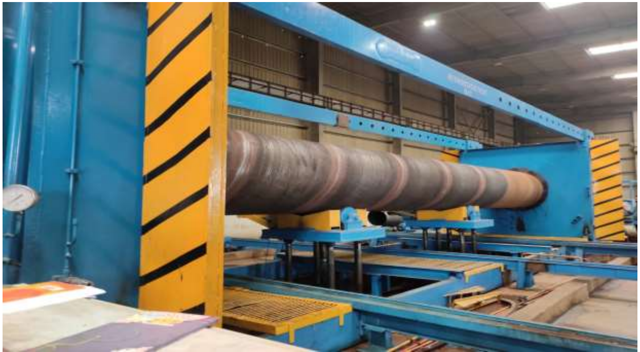
Figure 5.21: Hydrostatic Pressure test for pipe.
